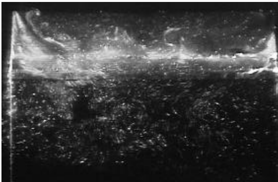
Figure 12 – Flow field adjacent to the hatch panel in a light sheet of 1 mm thickness parallel to the panel. View from behind in the upstream direction.
