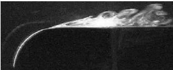
Figure 5 – Side view of the flow structure in the separation zone (middle plane). Vortical structures of the Kelvin-Helmholtz type are visible.
